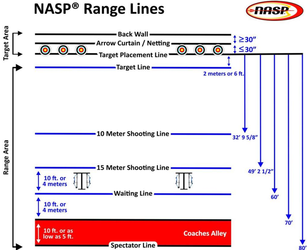
A NASP® range requires 80' of depth and 5' of width for every lane of a tournament. ***Each archer must have 30" of space in their portion of a lane.***
